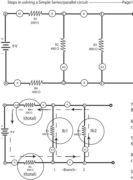
Think about the flow of electron (current) in the circuit it flows counter clockwise on this example.
