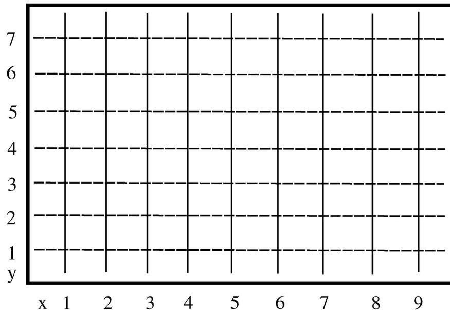
Fig. 3. The sensor construction of the rug showing the triggers running the length and width of the carpet creating a grid of x and y coordinates.
