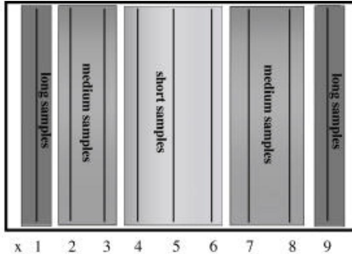
Fig. 16. The mapping of the x-sensors places control over longer sample lengths at the edges of the carpet.
